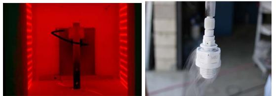
Photo on left shows a high-temp accelerometer on stinger test in thermal chamber at 1200°F (649°C). Photo on right shows a cryogenic pressure sensor after soak in liquid Hydrogen at -420°F (-251°C)
