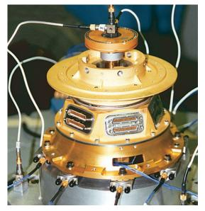
Vibration Measurements on an Atmospheric Infrared Sounder (used on Earth Observing System)
