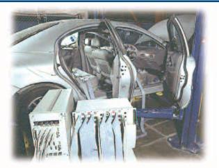
The 16-channel signal conditioner modules can be used to power large arrays of ICP<sup>®</sup> accelerometers, force sensors, pressure sensors, and microphones. These modules are an excellent choice for multi-channel NVH testing, acoustic array measurement, modal analysis, and GVT testing.
