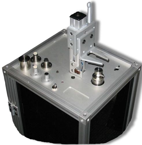
**Figure 9. Pneumatic shock test apparatus.** This device was used to take the amplitude linearity data shown in Figure 7. It was described in reference [2], and provides shocks from below 100 G to 10000 G for comparison calibrations tests. Tests through the full scale range and through to the levels at which the stops were engaged were performed on a Hopkinson bar.
