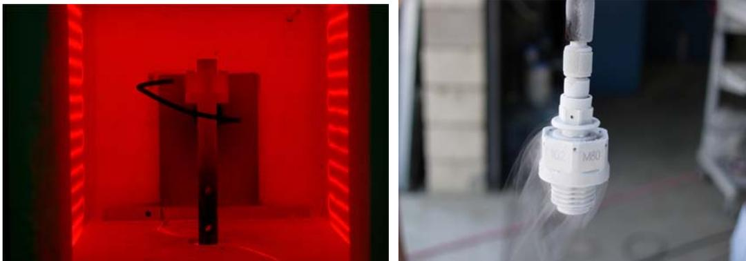
Photo on left shows a high-temp accelerometer on stinger test in thermal chamber at  $1200^{\circ}\text{F}$  ( $649^{\circ}\text{C}$ ).
