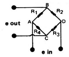
A regulated 5 to 20 volt DC or AC rms excitation is required and is applied between A and D of the bridge. When a force is applied to the transducer structure the Wheatstone Bridge is unbalanced causing an output voltage between B and C which is proportional to the applied load.
