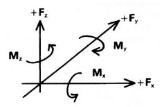
A "+" sign indicates force in a direction which produces a "+" signal voltage and generally defines a tensile force.
