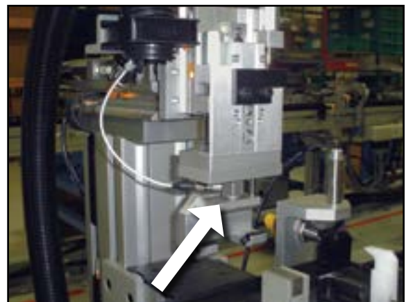
Assembly force monitoring using 208C Series force sensor
