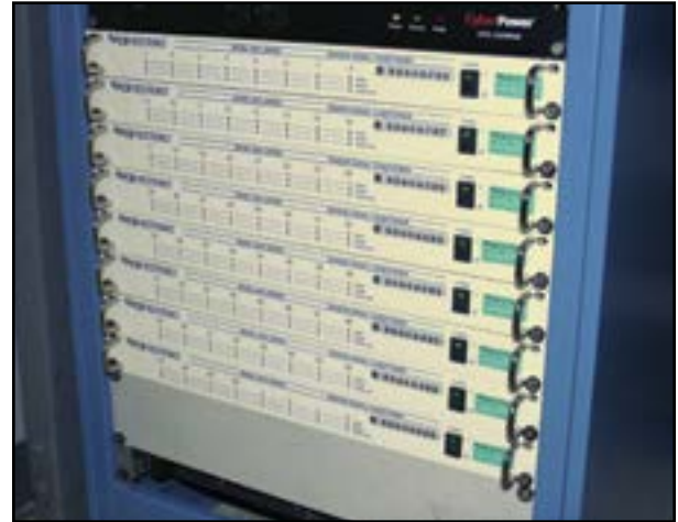
ICP® signal conditioners for 64-channel product modal test
