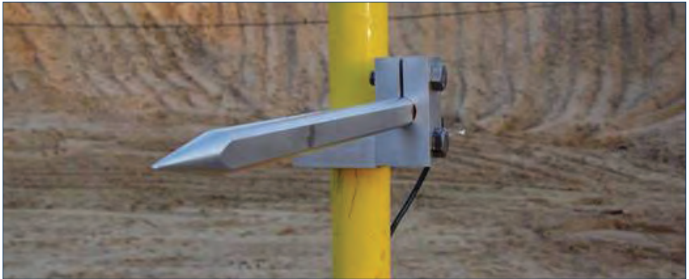
Photo 2: Typical mounting of a Pencil Probe.
