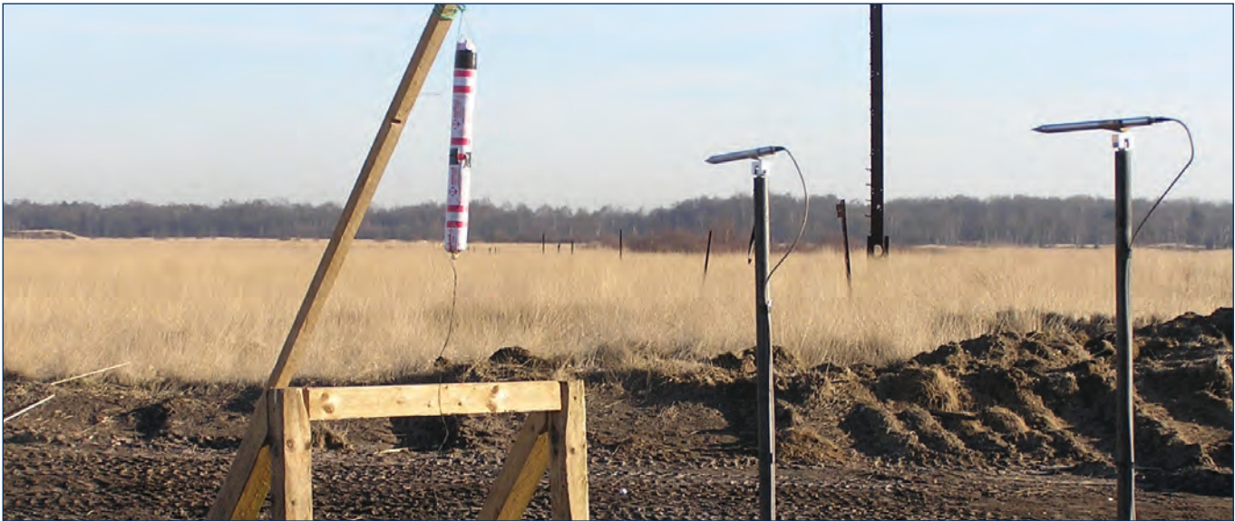
Photo 1: Pencil Probes are often mounted in multiple locations from the blast source.
