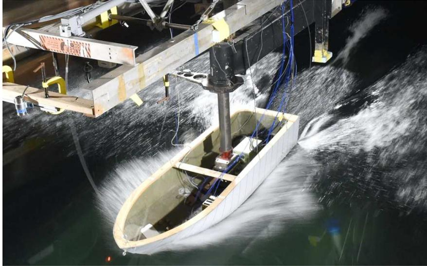
**Figure 1: Typical Open Tunnel Water Test of Ship Hull**
