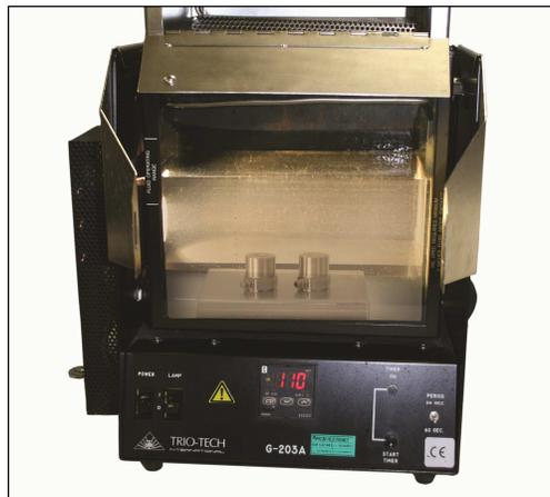
**Figure 8: Gross Leak Test Apparatus**
