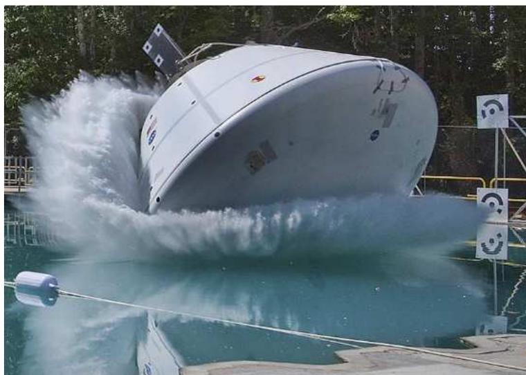
**Figure 4: Orion Crew Module Drop Test**
