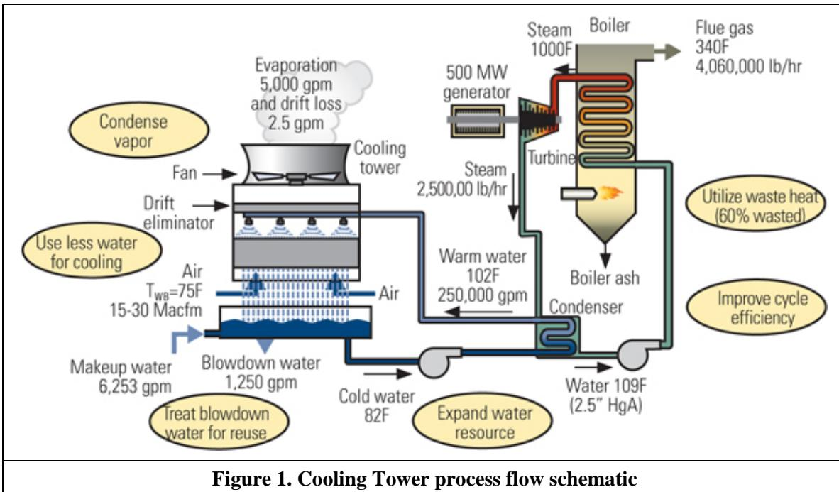
**Figure 1. Cooling Tower process flow schematic**
