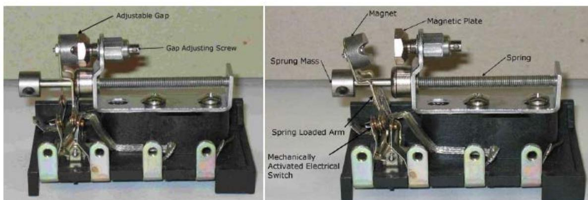
**Fig. 6(a) Armed mechanical switch mechanism with labeled parts**
