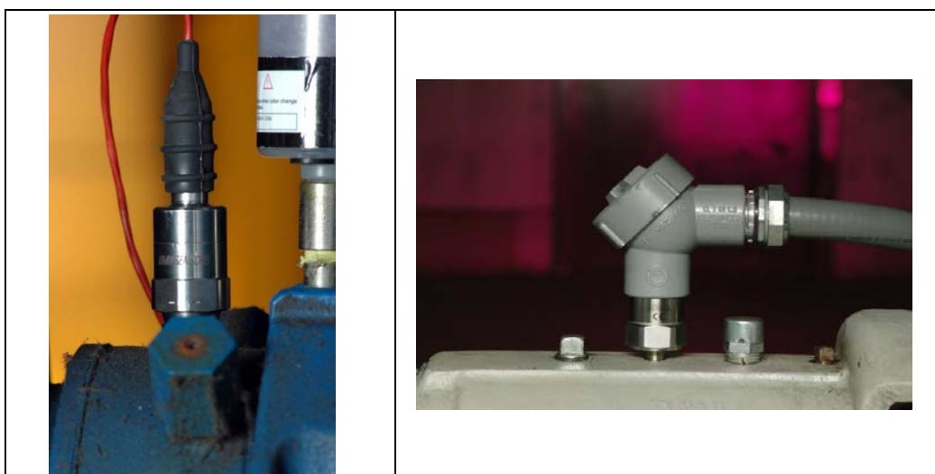
**Figure 10 SMART Vibration Switch mounted on a machine casings**
