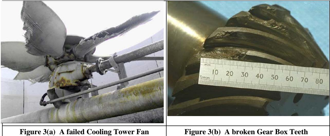
**Figure 3(a) A failed Cooling Tower Fan**
