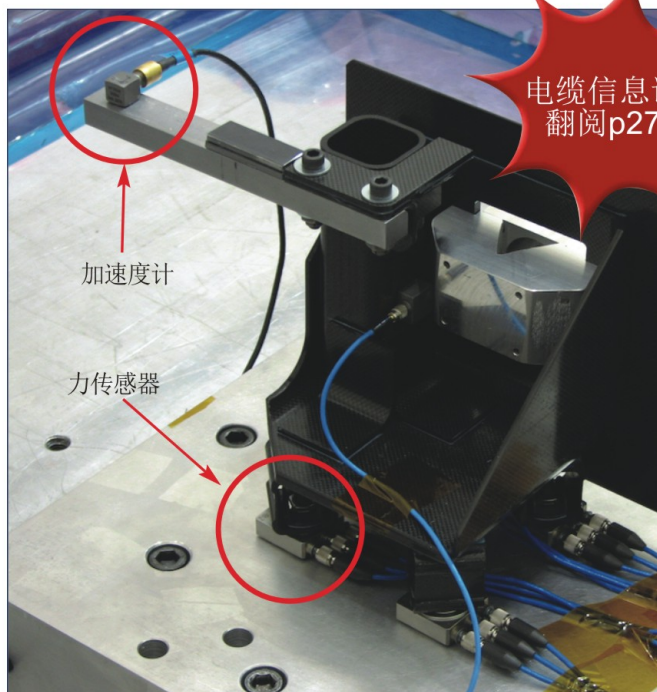
PCB® Model 356M208 accelerometer & force sensors used during vibration testing of bracket assembly at Utah State Space Dynamics Lab
