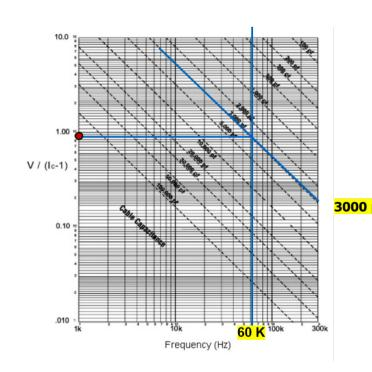
For ICP® sensors, the cable capacitance can introduce slew rate limitations at high frequencies and high voltages.
