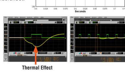
■ A maximum output of -229 mV was recorded, corresponding to only 3.9% of full-scale range
